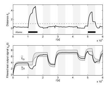
Fig. 9. Results of the fault detection with INFUMO3
