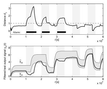
Fig. 7. Results of the fault detection with INFUMO1
