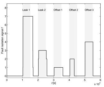
Fig. 10. Results of the fault isolation with a bank of INFUMOs
