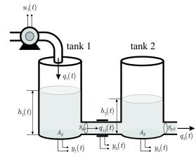
Fig. 2. Two-tank laboratory plant
