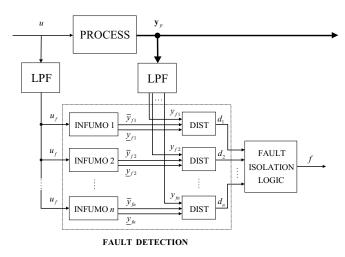
Fig. 1. Fault-isolation system using INFUMO models for FD
